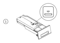
To remove the dispenser drawer from the washer, pull the dispenser drawer open, push down on the tab to the left of the MANUAL DOSE compartment and pull the dispenser drawer out from the washer.
