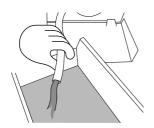
Unhook the pump outlet hose and pull it out (approximately 150mm). Remove the plug and allow any water (approximately 250ml) to drain into a shallow dish.
